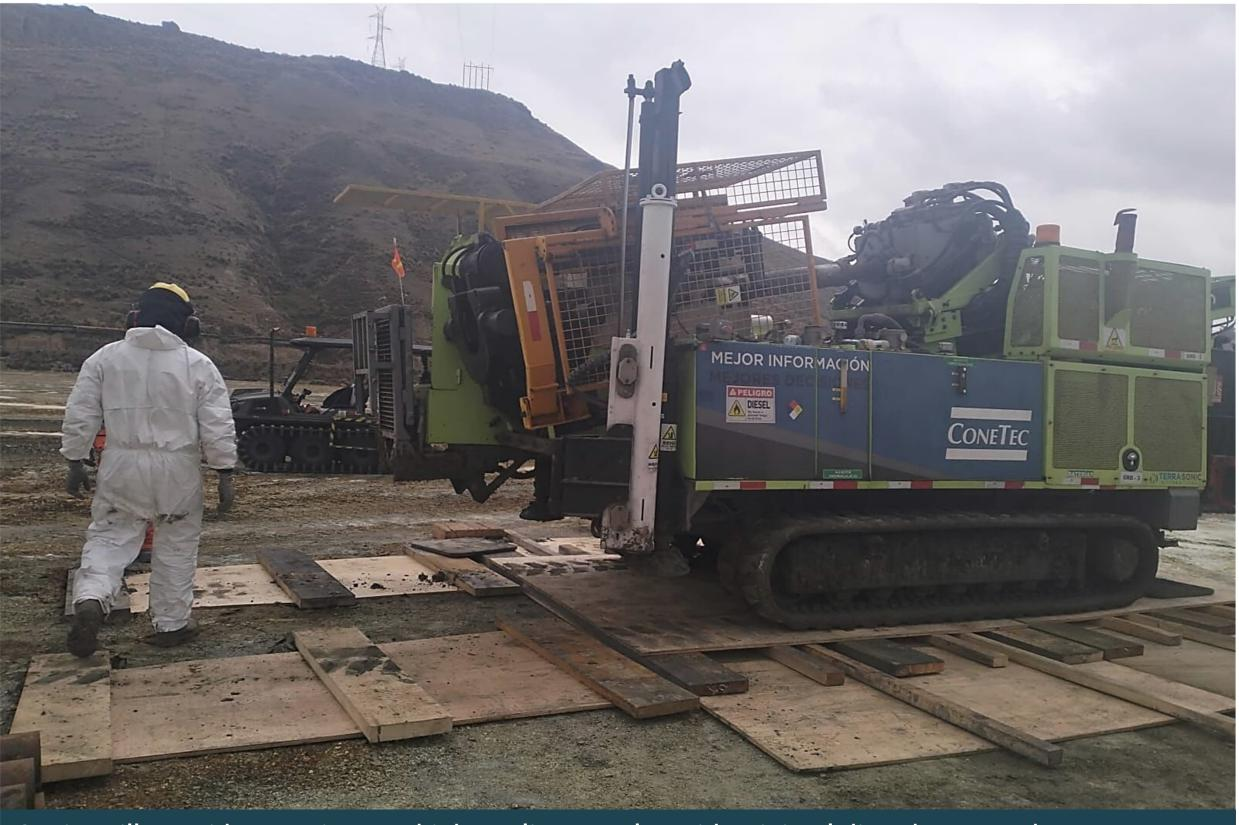
Sonic Drill, provides continuous, high-quality samples with minimal disturbance and no water usage, reducing environmental impact, enhancing resource recovery, and improving data quality.
