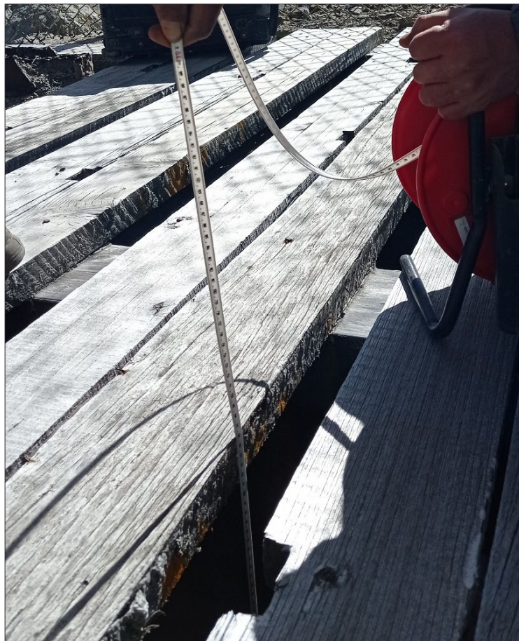
Figure 16-17: Measuring the water level at the La Cuiñada shaft
