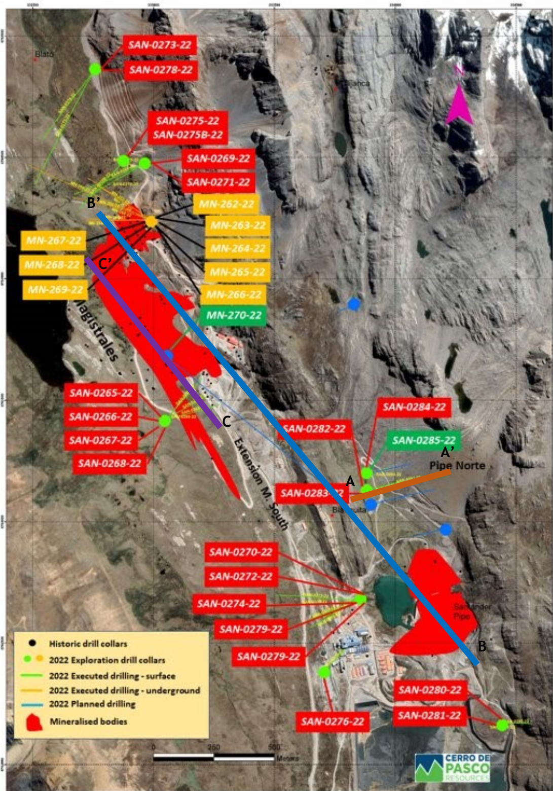
Figure 2: Plan view of Magistral and Santander Pipe mineralized bodies and drilling program executed to date
