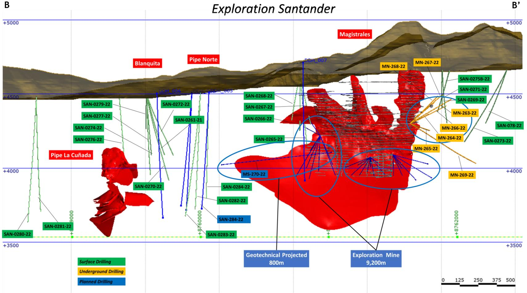
Figure 3: Cross-section showing executed and proposed surface and underground exploration boreholes
