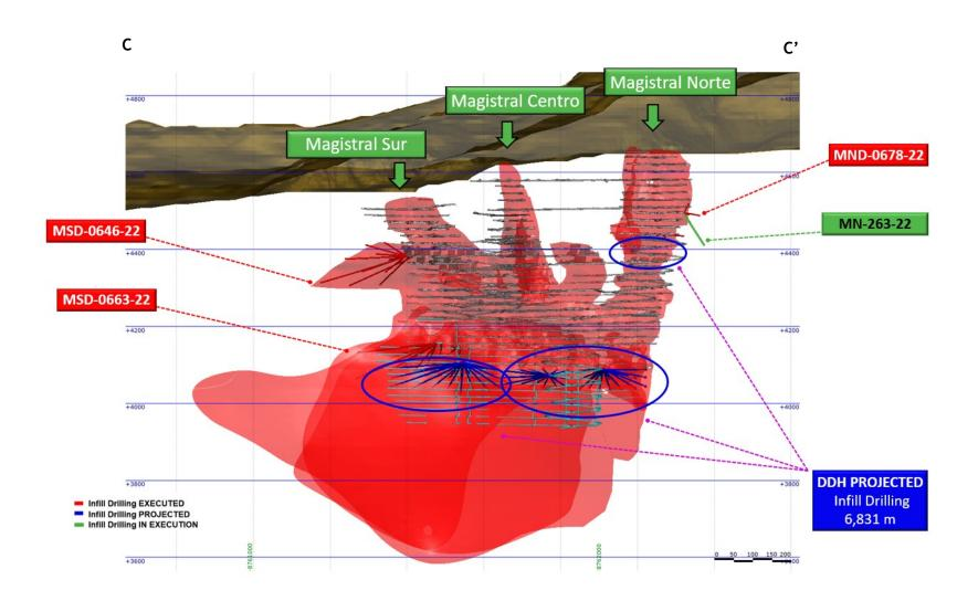
Figure 4: Infill drill program with drilled and programed holes
