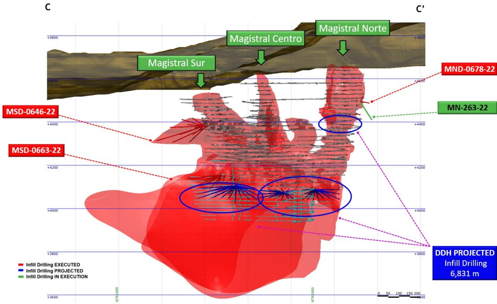
Figure 4: Infill drill program with drilled and programmed holes
