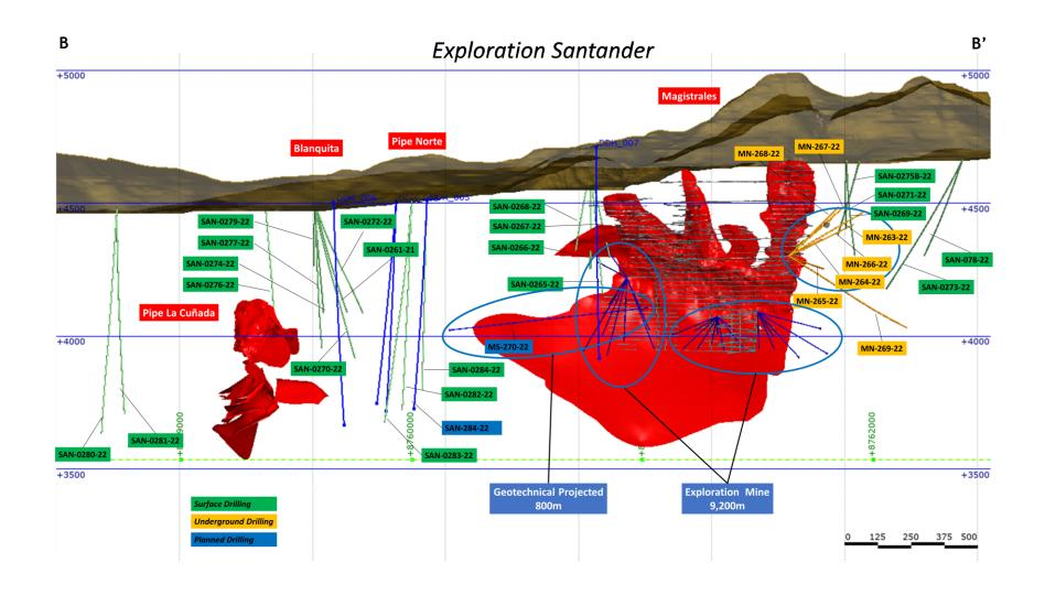
Figure 3: Cross-section showing executed and proposed surface and underground exploration boreholes
