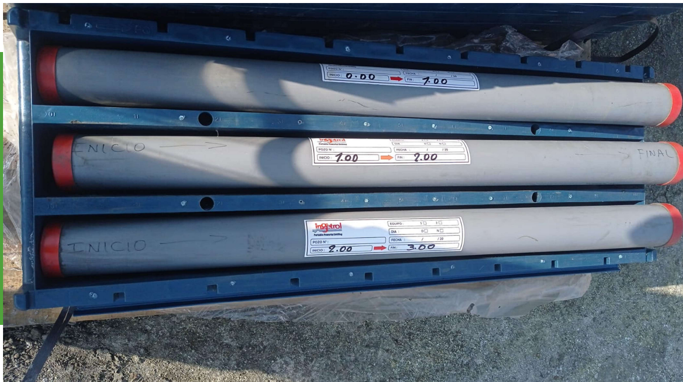
First drill samples from Quiulacocha Tailings ready for shipment to Bureau Veritas
