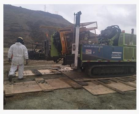
Sonic Drill, provides continuous, high-quality samples with minimal disturbance and no water usage, reducing environmental impact, enhancing resource recovery, and improving data quality.
