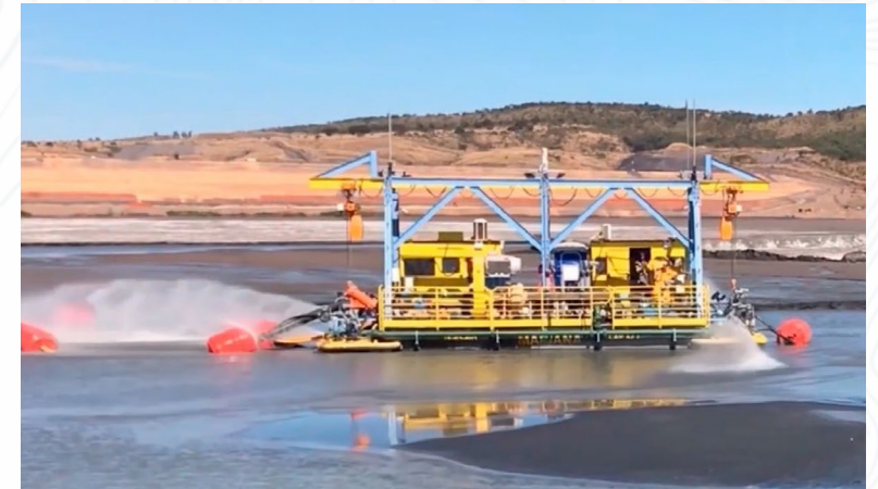
Example of Pump Pontoon for Tailings Extraction
